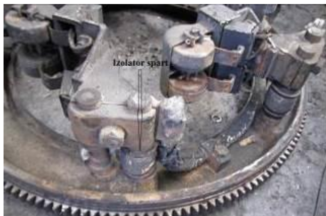
Fig.5 – Izolator spart
